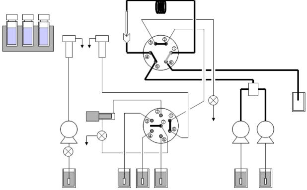
Mobile phase flows from the other side (originally connected to the high-pressure valve) of the outlet tubing. Collect it in a beaker or similar container.
