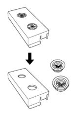
CAUTION: Potential System Damage. Make sure that the caps are fully installed. If they are loose, they might touch the Z mount.
