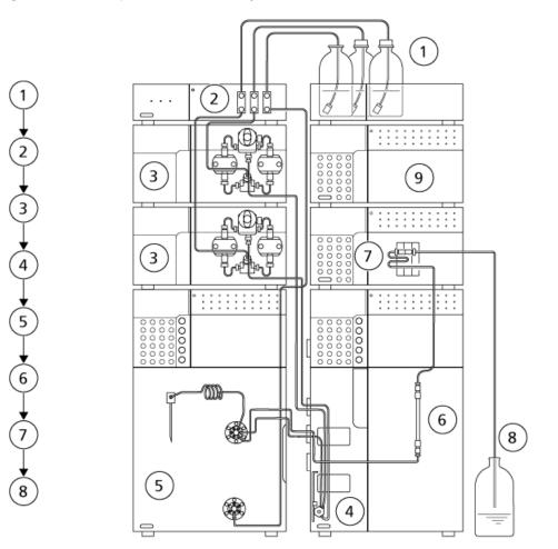
Figure 3-1 Example ExionLC AD System
