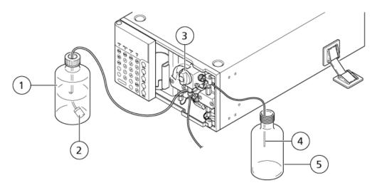
2. To open the drain valve, turn the drain valve knob 180 degrees counter-clockwise.
