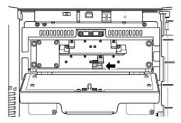
3. Confirm the direction of flow for the column, and then connect the outlet tubing from the pre-heater to the column inlet. Use the UHPLC fitting attached to the oven.
