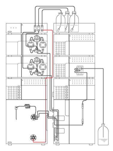
Figure 6-4 Plumbing for High-Pressure Gradient System
