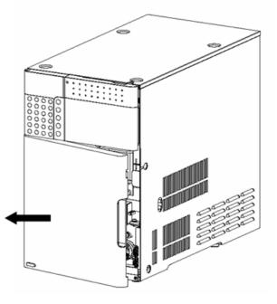
Figure 5-40 Opening the Autosampler
