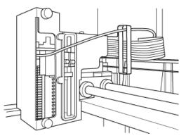
7. Route the new sample loop through the square hole at the back of the Z mount, and then insert it through the positioning hook on the right side of the Z mount.
