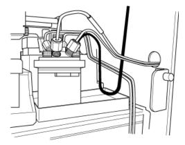
Figure 6-27 Tubing Routed Along the High Pressure Valve
