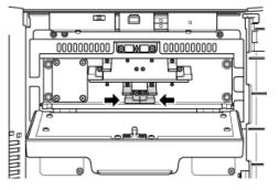
Figure 5-6 Column Block Position, 60 mm to 120 mm Column
