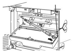
Figure 5-9 Connecting the Column Outlet Tubing
