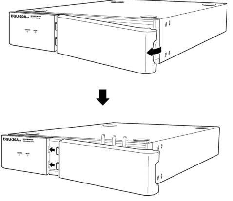
2. After connecting the tubing, replace the front panel to protect and to fix the tubing connectors. Align the two lugs at the left of the front panel with the recesses in the unit.
