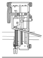
CAUTION: Potential System Contamination. Insert the needle fully into the connection, then tighten with a wrench. If the needle is not inserted fully in the hole, a dead volume is created resulting in peak diffusion or cross-contamination.
