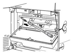
4. Connect the tubing from connected to the detector to the column outlet.
