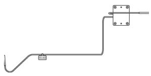
6. Insert the bent end of the outlet tubing (the end with the identification tag) through the round hole in the side panel of the autosampler.
